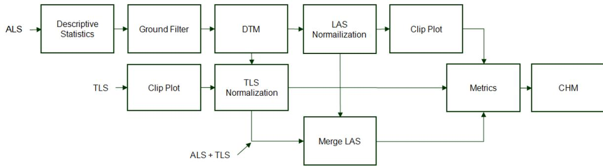
Figure 2. Flowchart for processing and merging the LiDAR data to arrive at individual and combined CHM.
