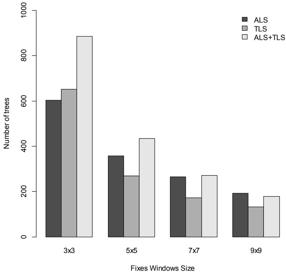
Figure 4. Number of the trees detected from the LiDAR CHM using the Web-LiDAR Treetop application
