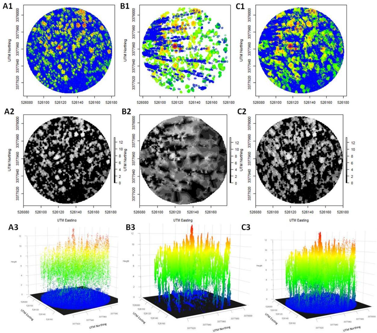
Figure 3. The static plot view, canopy height model (CHM), and 3D point cloud for ALS (A1-3), TLS (B1-3), ALS+TLS (C1-3).
